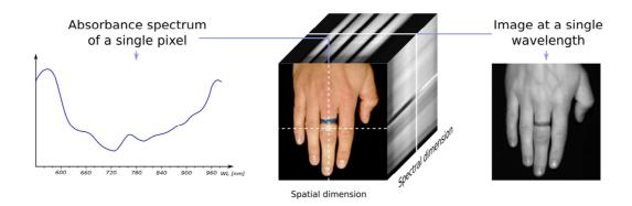
In Hyper Spectral Imaging (HSI) Technology three dimensional ( X [spatial], Y [spatial],  $\lambda$  [spectral] ) data cubes are generated. Based on the data cubes different images and chemical information can be extracted.
